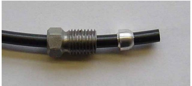
Make sure that the clamp-seal-ring has the right direction! See picture
