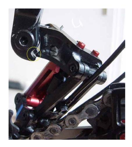
**3.** Remount the rear wheel. Mount the chain (if you prefer to remove the upper pulley of the derailleur, instead of opening the chain: The pulleyscrew uses a torx20 key; Please check the length of the chain carefully, massive damages can occur especially with a full suspension frame, when the chain length is not correct).
