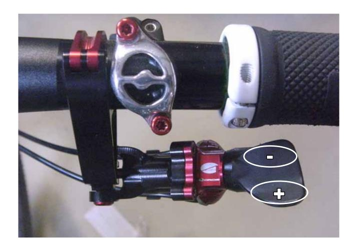
Push the shifter in its upper area to shift to a smaller cog-ring or chainring. Push the shifter in its lower area to shift to a bigger ring (the handle plate swivels under your finger to change the internal valve position).
